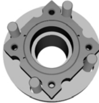
Figure 3 SRB-7RS™ Safety Head Companion Flange Bolting Pattern (Capscrews removed for clarity)
