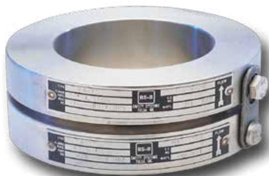
BS&B Quik-Sert safety head - flanges are assembled with bolted side lugs in sizes through 8 inches ID - with recessed cap screws in 10 inch size and up
